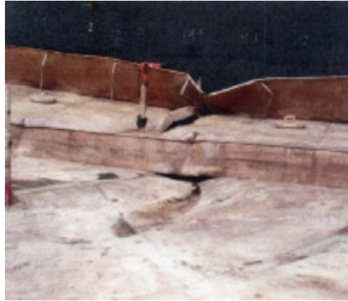
Image 4: Pontoon buckling [Tetsuaya, 2007]
